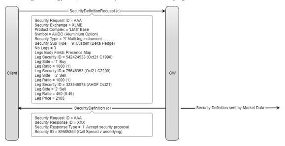
A denominator of 1000 is applied to the Leg Ratio value which is shown in brackets.
